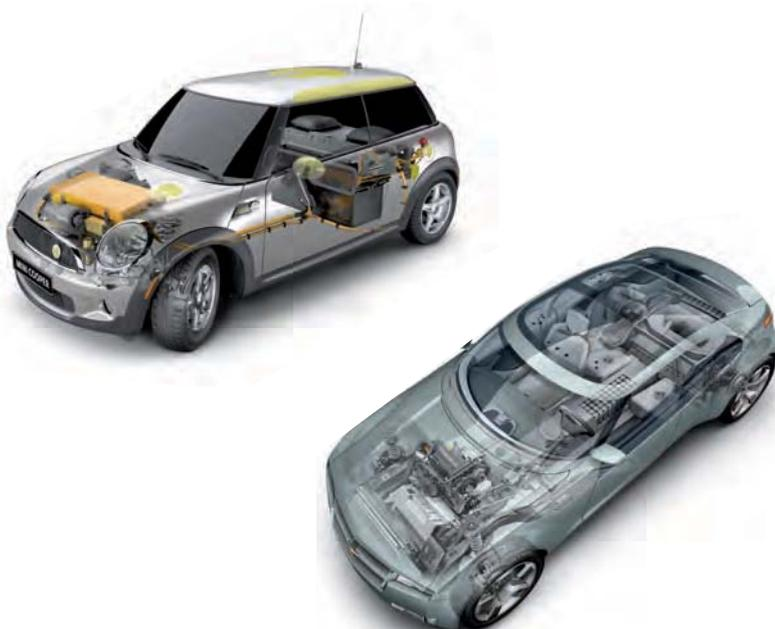
Abbildung 14: Conversions-Design (BMW-Mini) vs. Purpose-Design (Chevrolet Volt)<sup>31</sup>
